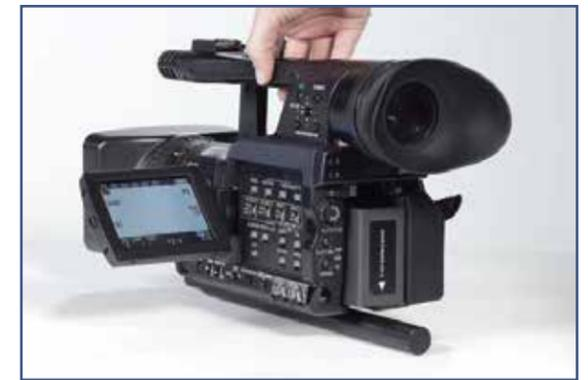
Rotate the camera 90° and find the **Side-to-Side** balance point. When found, mark the point on the camera using a piece of tape.
