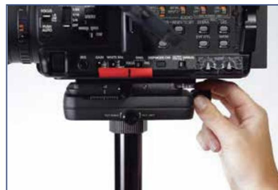
Use the **Fore-and-Aft Adjuster Knob** to balance the **Post** vertically.
