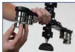
Fold out the **Wings** and add **Balance Weights** as recommended in the chart below.
