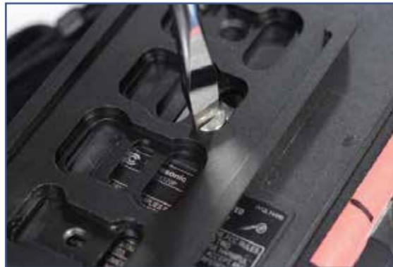
Fasten the camera to the **QR plate** securely with the appropriate camera screw. Ensure the **Fore-and-Aft** and **Side-to-Side** balance points are centered on the plate with the lens parallel to the plate.
