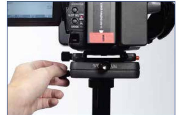
Using the **Side-to-Side Adjuster Knob**, align your **Side-to-Side** mark with the **CENTER** of the Post.
